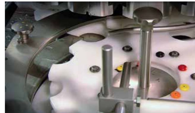
▲ Heated product bowl with 2 hinged access doors allowing easy access to the bowl for inspection and cleaning.
