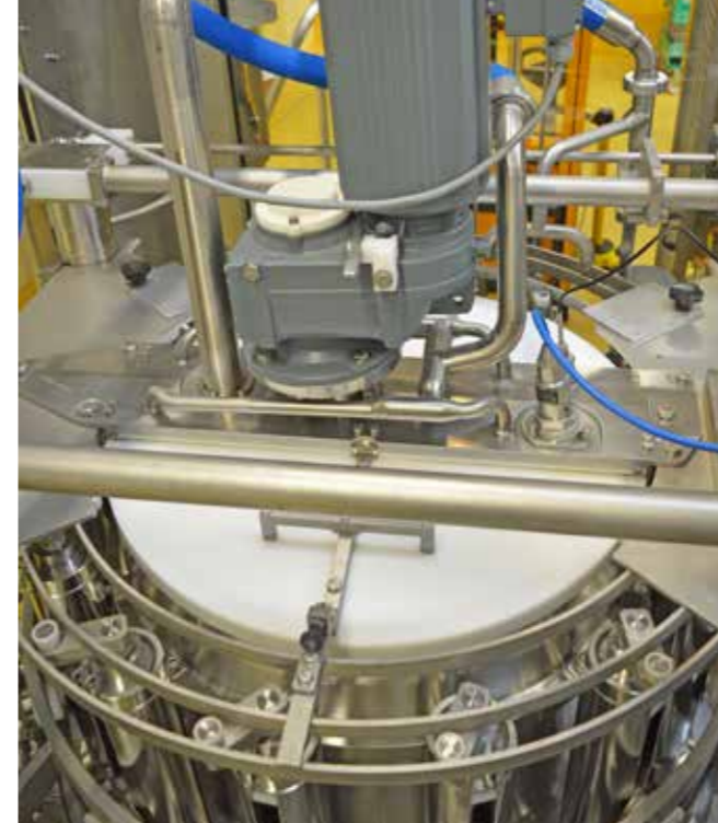
▲ Heated product bowl with 2 hinged access doors allowing easy access to the bowl for inspection and cleaning.
