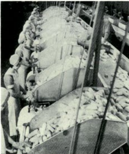
(Top) Major shippers of fresh tomatoes relied on the Cutler Weight Principle Sizer that sized fruit by weight.
