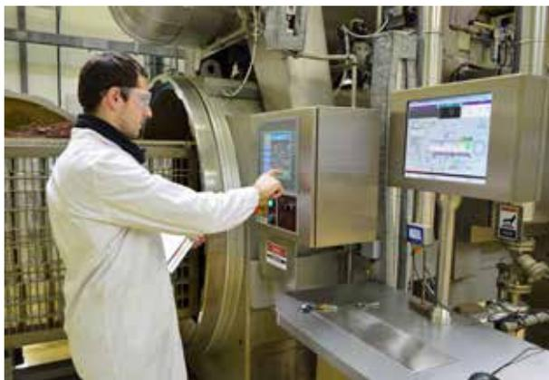
For JBT, a well-performing in-container sterilization system relies on an advanced processing principle with a unique sterilization control system that provides a consistent, optimal and efficient thermal processing system under full management control.
