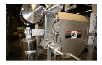
The Prime Paw Cutter is a high-volume, efficient and durable solution to remove the shank from paws. Mounted in-line, the Paw Cutter removes the shank with a rotary blade, while two brushes capture the paw and remove it from the shackle once the shank is cut. Made of high-quality stainless steel and built to last, the Prime Paw Cutter is part of a complete paw processing system.
