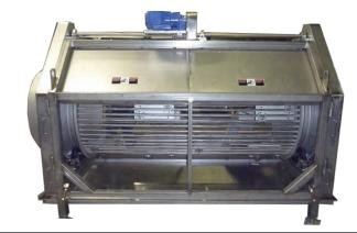
Prime BT-Series Bird Tumblers are designed to remove excess water from beneath the skin of birds, typcially after chilling. With stainless steel construction, a 38-inch diameter rod screen and dual 3-hp drives, BT-Series Tumblers safely and effectively tumble birds without damage.
