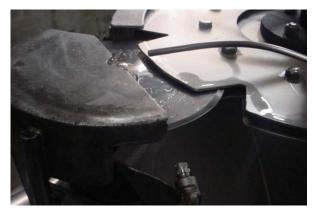
The WLNSC-1 Wing Lift Neck Skin Cutter is a line-driven solution for removing necks from chickens in the evisceration or cut-up areas. This machine is specifically designed to divert wings from the neck-cutting blade to preserve wing quality and yield. The WLNSC features an indexer to hold birds in place and is line-driven.
