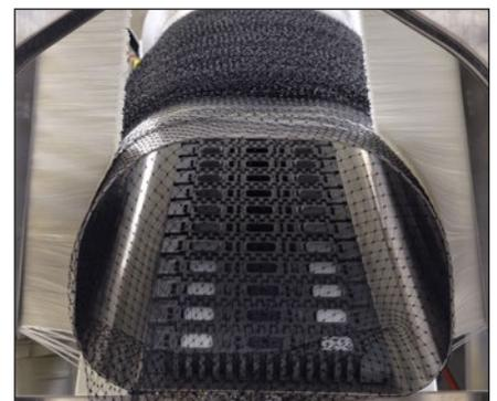
Optional roller belt inside horn assists products through the chute.
