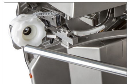
Quick-release casing brake design for fast casing changes.
