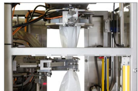
Hands-free automated filling and clipping for reduced labor requirements.
