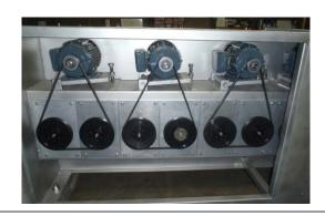
The Prime RP-3000 Counter-Rotating Picker utilizes the most effective and versatile defeathering method available. The first opposing drums pick downward; the next pick upward, for maximum picking success. This innovative method allows lower scalding temperatures. Also, the skin remains more firmly attached to assure a product of higher grade and yield, with better appearance and value.
