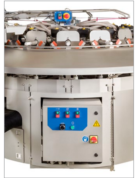
Simple, highly visible control panels make it easy to manage vital functions like start/stop, vacuum pump, rotating product table, and bag tail takeaway.
