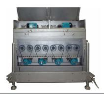
The Prime RF-6 Counter-Rotating Picker utilizes the most effective and versatile defeathering method available. The first opposing drums pick downward; the next pick upward, for maximum picking success. Additional banks of picking drums focus on hocks at the same time. This innovative method allows lower scalding temperatures. Also, the skin remains more firmly attached to assure a product of higher grade and yield, with better appearance and value.
