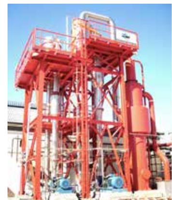
Compact Hot Break enzyme inactivator and TFCE 1E-1S-3 Evaporator
