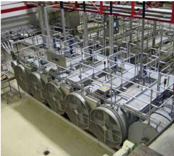
Practice makes perfect. 90% of the world's production of canned evaporated milk is sterilized on JBT's Continuous Rotary Pressure Sterilizers.
