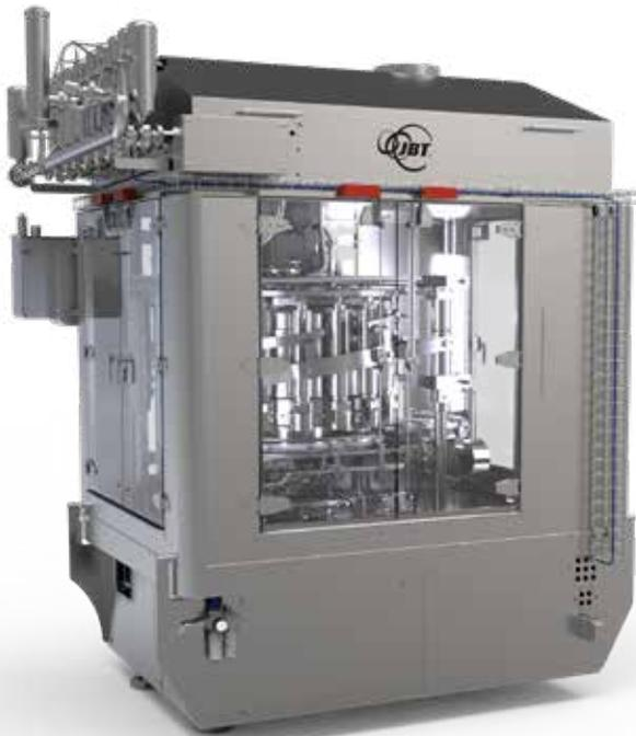
For dairy applications, these unique Unifiller features deliver the following key benefits (i) superior fill accuracy with minimum give-away and consistent headspace, (ii) fully automatic cleaning in place (CIP) without fill station disassembly and (iii) the flexibility to fill products with or without particles.
