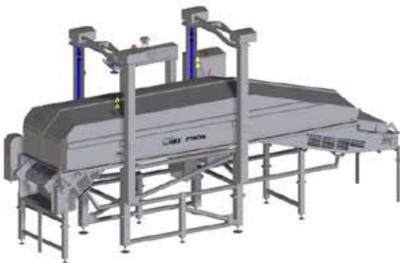
Example of the DCC Belt steamer, type single belt system. In the right figure the hood is in cleaning position. The inner side of the hood and the whole belt are easy accessible for cleaning.
