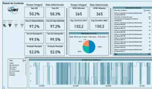
The main iOPS® dashboard contains high level key performance indicator statistics for measuring OEE, Availability, Productivity and more. Click on any of the information buttons on the main dashboard to drill down to detailed granular KPI data. All dashboards generate reports and filter by date ranges, with drill down by
