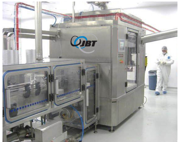
▲ JBT SeamTec™ Pre-gassing Closer with gas-tight guarding
