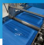
Machine redesign facilitates easy removal of the non-modular belt to make sanitation and maintenance more efficient
