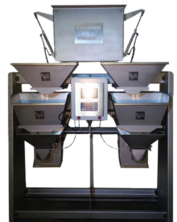
Baggers/Scales with JBT Controller
