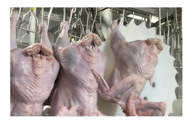
The Prime Equipment Group Rotary Bird Unloader is a simple solution for removing birds from the shackle at any point on the line. The chainless deisgn eliminates broken or damaged hocks caused by chain binding, and its simple design is easy to clean and maintain.
