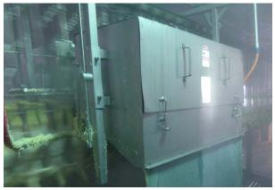
The HP-3 Hock Picker is a simple, effective and proven solution to remove hock feathers quickly and efficiently. Designed with three rotating heads per side, its simple design makes maintenance and sanitation easy.
