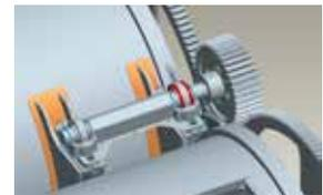
For better performance and less maintenance the single, longitudinal shaft is nowadays replaced by drive motors and counter shafts directly placed on the bull gear.
