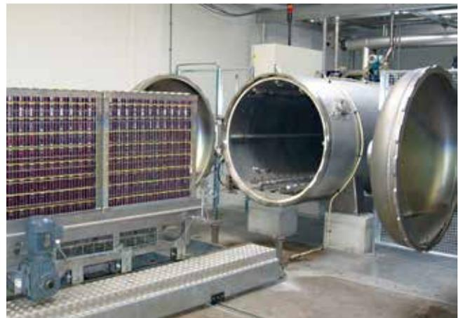
Transport system using a shuttle
