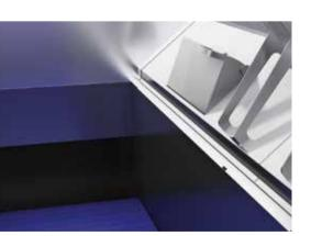
By fine-tuning airflow through the product bed, the air bypass ensures gentle, optimized fluidization regardless of product shape, size and weight. It also helps to maximize heat exchange over the evaporator, and minimize over-blow of light products.
