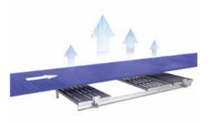
By modulating airflow on the first IQF Track, you can fine-tune initial crust freezing to the exact requirements of each product and eliminate product 'clumping'.
