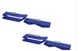
To ensure proper IQF at the critical crust-freezing stage, back-and-forth agitation on the first track or on your tray separates long or sticky products like sliced bell peppers, pasta, onion rings and rice. Stepless speed adjustment on both conveyors also helps increase your throughput of staple IQF products like peas, beans and cauliflower.
