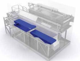
The IQF Track offers stable, dual zone fluidization, with two independent tracks and two separate pressure chambers. Crust-freezing for stable IQF, appearance and yield, and then fresher-than-fresh core freezing, it can be run in either agitation or conveyor mode, ensuring optimum IQF for both delicate and hard-to-handle products.
