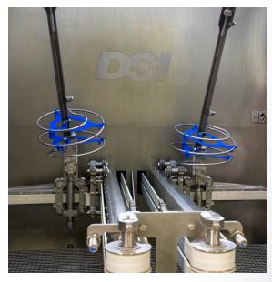
DSI portioning systems that run as high as 87,000 psi require a delivery system with stainless steel coils that were specified for their high strength and reliability. Your 60,000 psi unit with a high pressure hose delivery system may now be upgraded to these stainless steel coils to improve wear and minimize maintenance.
