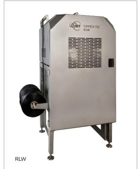
uses wheels instead of grippers to hold and move netting, the RLW model is more accommodating to triangular or similar shaped horns. It handles extruded nets and loose weave style nets that are less elastic. The rucker works with chute sizes up to 14 inches (355.6 mm). Both the chute type and size are flexible and adaptable to other types and sizes.
