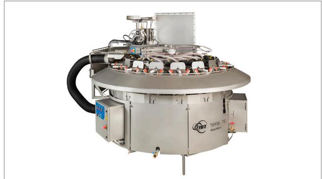
Rota-Matic automatic vacuum packaging system for whole birds, pork shoulders, ground meat chubs, rings, loaves, hams and cheese. Operates at speeds up to 40 packages per minute, with 8 or 16 stations.
