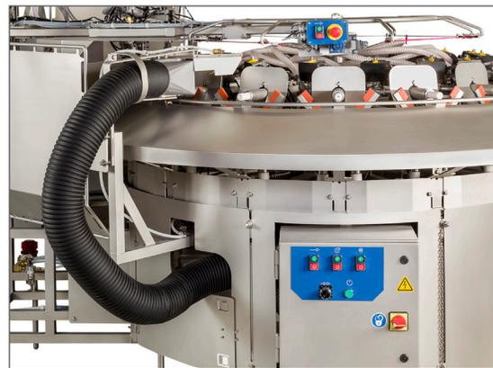
Simple, highly visible control panels make it easy to manage vital functions like start/stop, vacuum pump, rotating product table, and bag tail takeaway.
