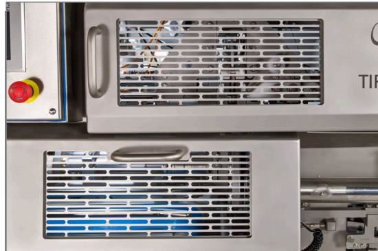
Optional Stainless steel window inserts can be ordered in place of the haze resistant Poly Carbonate
