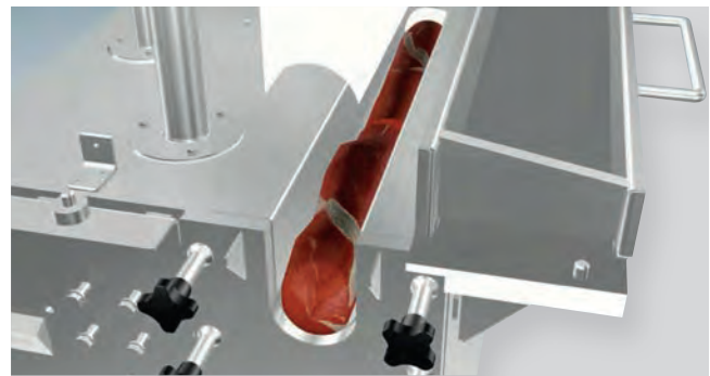
The meat is fed into the magazine using the sliding tray system
