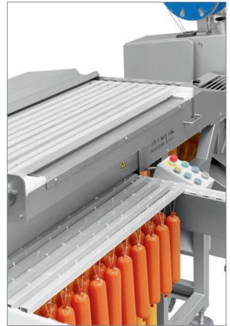
Motorized smoking stick magazine accommodates 22 smoking sticks.
