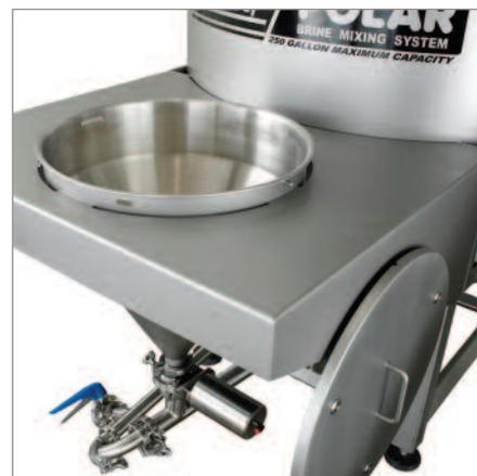
*The educator introduces ingredients directly into the liquid stream, allowing effective mixing without clumping.*
