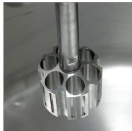
*The optional high shear mixer head provides powerful mixing options for challenging ingredients such as starches and gums.*
