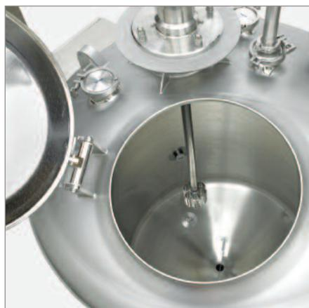
*All contact surface areas are highly polished, while the tank's outer walls are insulated and covered with a stainless steel shell to prevent condensation.*
