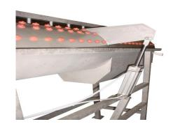
When used down-line from Prime's In-line Paw Scrubber (ILPS), the PPS-series Paw Scalder gains new efficiencies to reduce hot water usage and lower operating costs. In this application, the Paw Scalder serves as a final cleaning step after the ILPS. Therefore, water temperature in the scalder can be lower, preserving fat and increasing final product weight.
