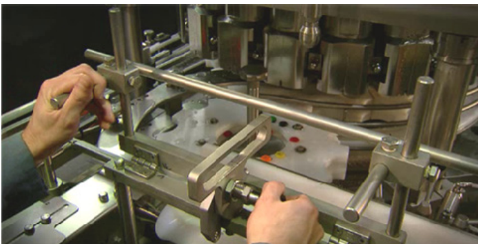
▲ Colour-marked Quick-change parts with locating pins for quick and correct positioning. ▼ Automatic height and volume adjustment
