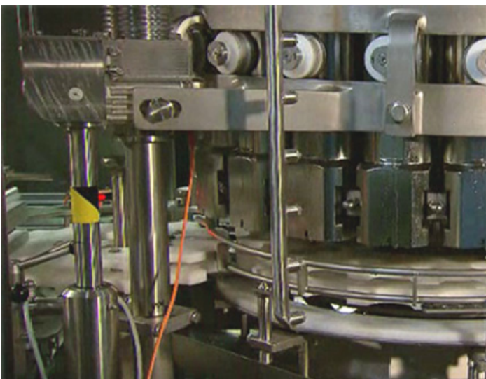
▲ Colour-marked Quick-change parts with locating pins for quick and correct positioning. ▼ Automatic height and volume adjustment
