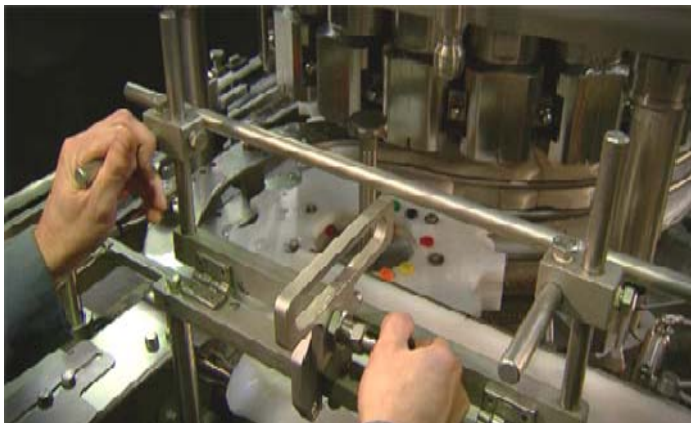
Color-marked Quick-change parts with locating pins for quick and correct positioning.
