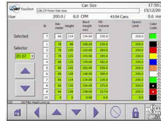
Machine display. 10 pre-set product-format combinations. Also change part colour codes are shown.
