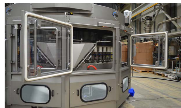
Mechanically and electrically locked side doors for easy access to the filling area of a Ultra Clean Precifill™
