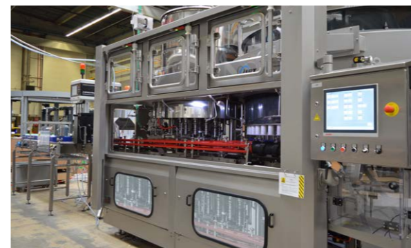
The Ultra Clean Precifill™ features an automatic side door for easy access to the infeed and capper unit
