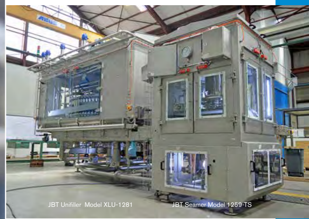
A JBT Unifiller XLU with 81 filling stations synchronized with a JBT 12-spindle seamer
