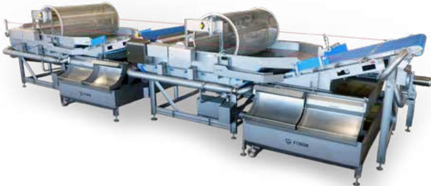
Flotation Wash Line for fresh cut salads, vegetables and herbs
