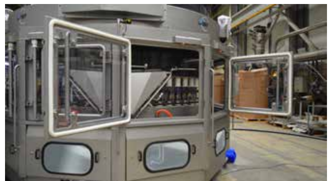
Mechanically and electrically locked side doors for easy access to the filling area of a Ultra Clean Precifill™
