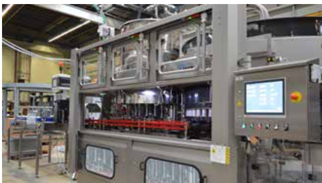
An automatic side door for easy access to the infeed and capper unit Ultra Clean Precifill™
