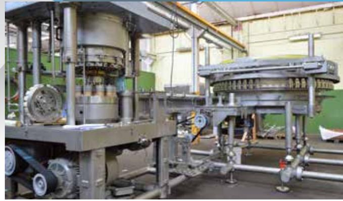
Complete machine rebuild of a 10-head X59 seamer synchronized with a high-capacity filler with 66 fill stations. Output 800 to 1200 cpm. Upgraded with full automatic lubrication and C.I.P. skid for dairy applications.
