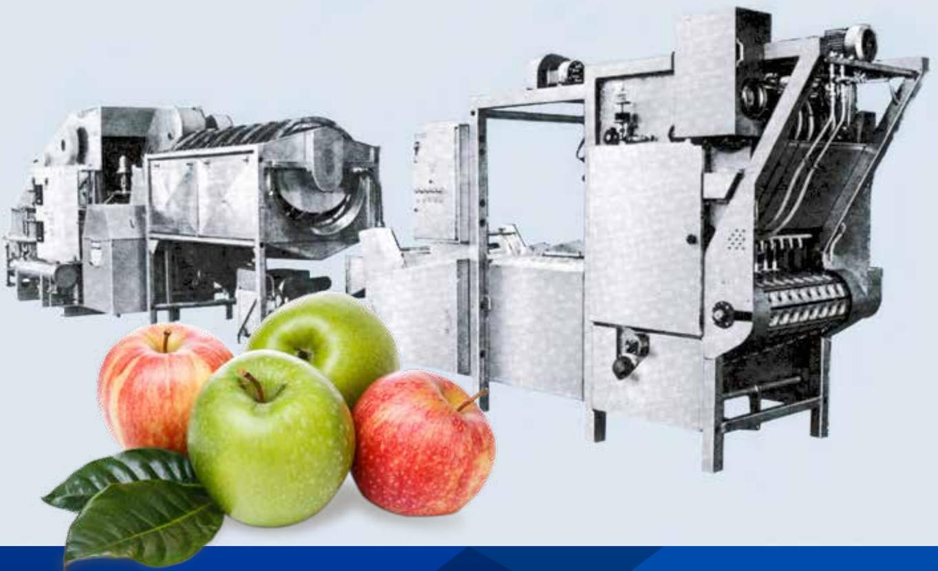
Designed to peel, stem, core and slice apples
