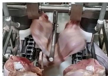
Breast cut from wings and dropped to conveyor
