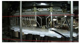
The Prime HM-2 Chicken Halving Machine automatically and effectively separates the front half from the saddle. Operating at speeds exceeding 180 BPM, the HM-2 can be adjusted to remove more rib bones or saddle to maximize leg quarter yield. The Halving Machine can be adjusted to completely cut front halves from the saddle or leave the front half hanging by the back skin, to be removed by the back skin cutter to maximize skin and fat yield.
