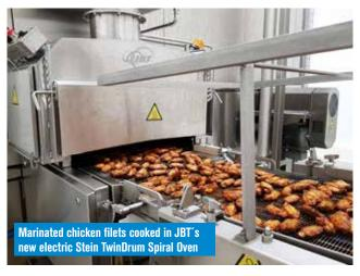
Even when JBT first developed the Stein TwinDrum Spiral Oven, they thought about using electricity as an alternative. However, the assessment was that the technical challenges of using electric power in hot and wet areas were significant. Therefore, it was initially designed only for heating by thermofluid. Based on Norsk Kylling's extensive requirements specification, JBT modified its basic design, making it their largest electric oven in Europe.
