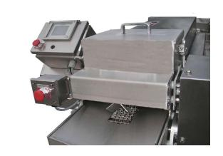
The CFS-TSK-1 Turkey Thigh Skinner Deboner effectively removes meat and skin from turkey thighs utilizing Prime's patented bladeless skinner and high-pressure water jets. Our CFS-Series units produce an open meat fillet ready for trimming, and our method of water jet deboning has been operating successfully across the U.S. turkey industry for more than two decades.
