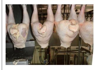
The BSC-1 Back Skin Cutter is designed to work with the HM-Series Halver to fine-tune the location of the skin cut between the front and back halves. This allows for extra yield to remain with either half. Additionally, the BSC-1 enables the front half to be dropped at a location downline from the halver for ease of product flow.
