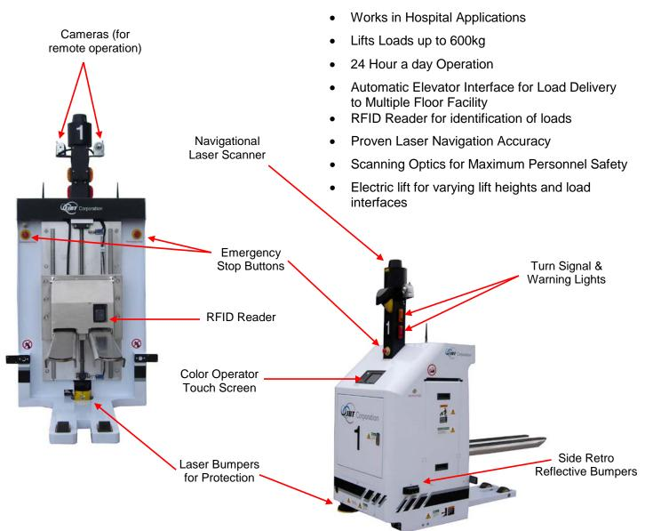
The ATLIS-F Laser Guided hospital vehicle is equipped with forks specifically designed for lifting hospital carts. Powered by an electric lift, these forks allow the vehicle to perform picks and drops by maneuvering the forks underneath the designated cart and actuating the lift mechanism.
