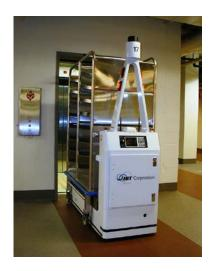
The ATLIS Laser Guided hospital vehicle is a unit load style vehicle with an integral lift mechanism, designed for lifting hospital carts. All picks and drops are performed as the vehicle's lift deck maneuvers under a designated cart, stops, and actuates its lift mechanism.
