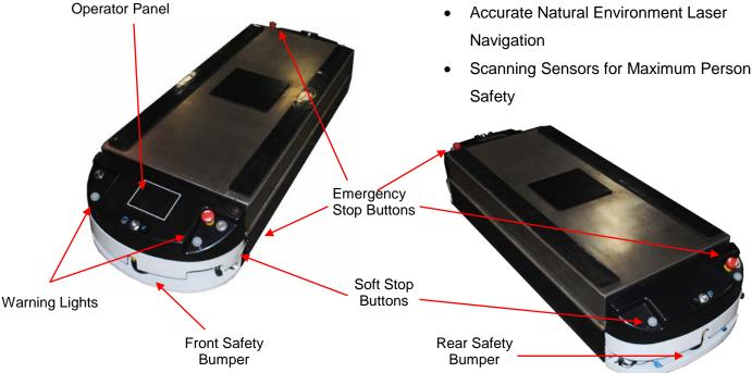
The ATLIS Laser Guided hospital vehicle is a unit load style vehicle with an integral lift mechanism, designed for lifting hospital carts. All picks and drops are performed as the vehicle maneuvers under a designated cart, stops and actuates its lift mechanism.
